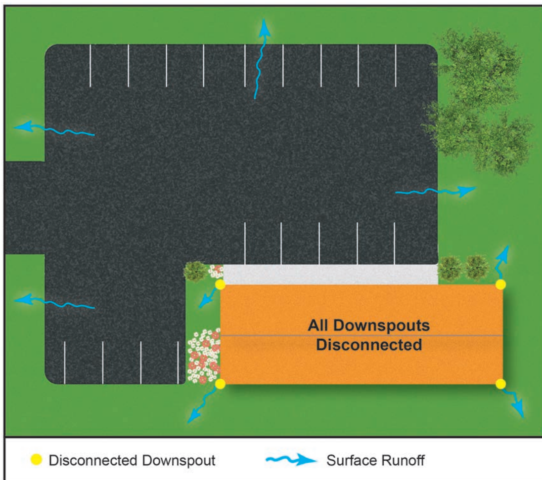
Figure 11: Disconnected Downspouts Draining to Pervious Area
