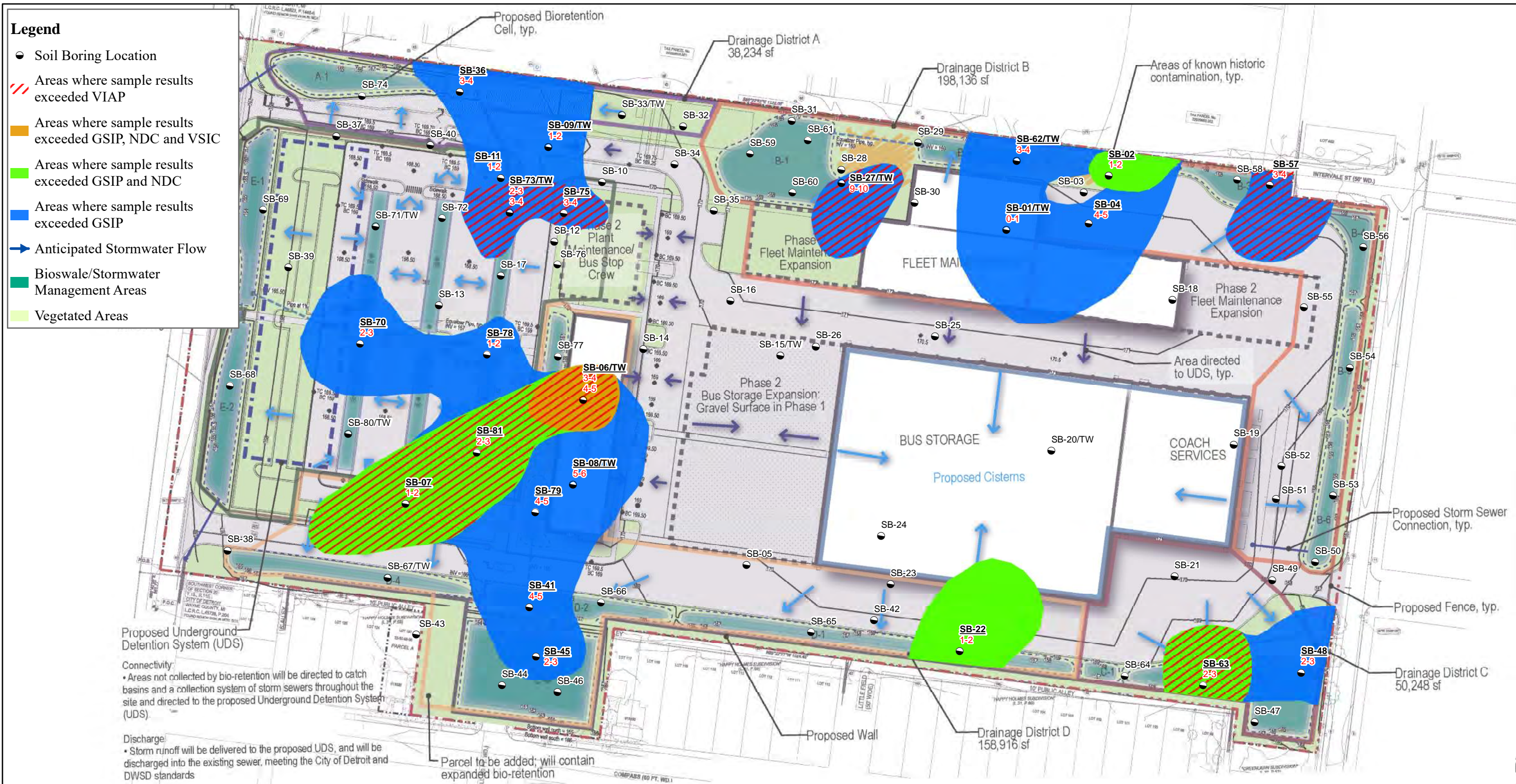
Figure 6 Semi-Volatile Organic Compounds in Soil Coolidge Bus Terminal 14044 Schaefer Hwy Detroit, MI 48227 Detroit Building Authority
