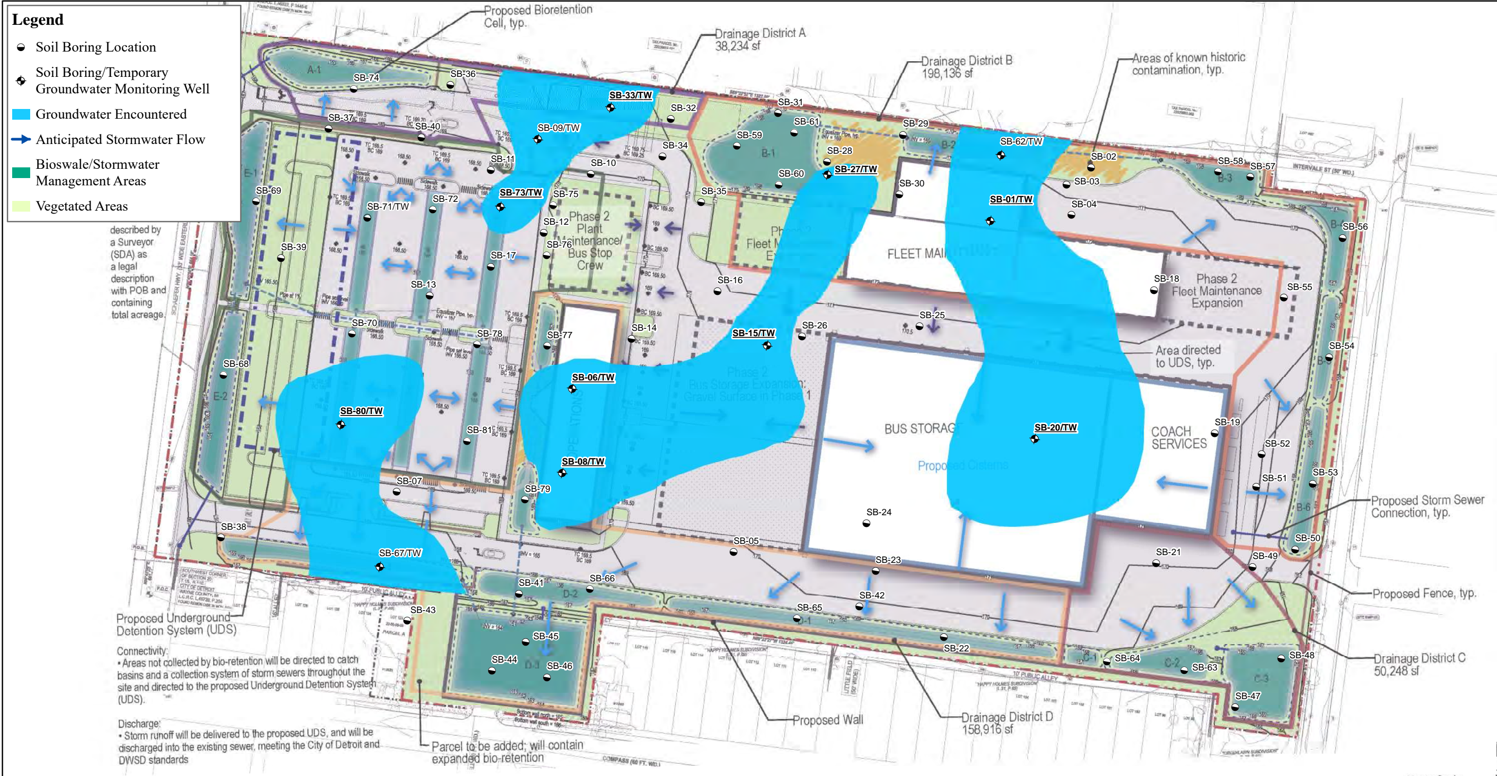
Figure 8 Groundwater Location Map Coolidge Bus Terminal 14044 Schaefer Hwy Detroit, MI 48227 Detroit Building Authority
