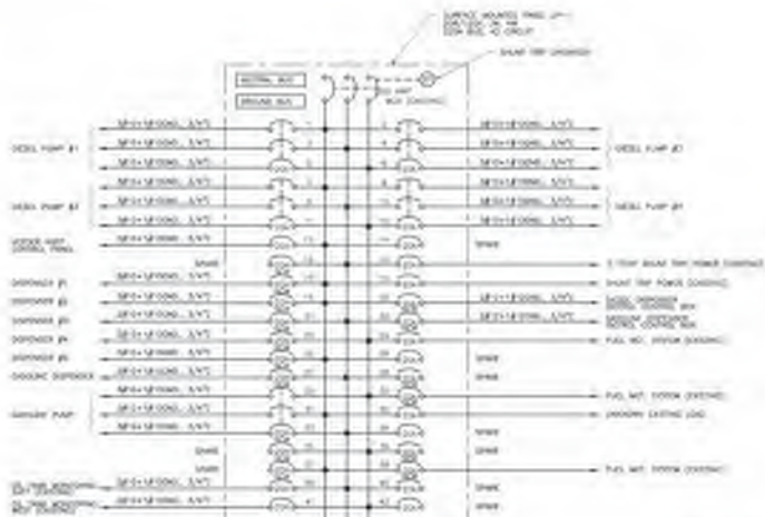
ELECTRICAL DISTRIBUTION DIAGRAM MULT-PUMP/MULT-FUEL NOT TO SCALE
